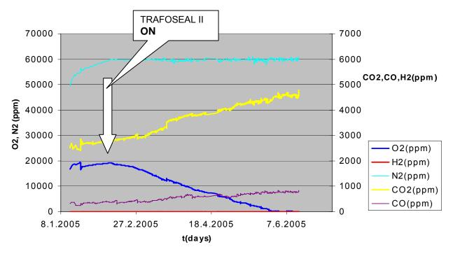
Fig.4. Dynamic of dissolved gases in oil of the main tank before / after switching the TRAFOSEAL **ON.**
