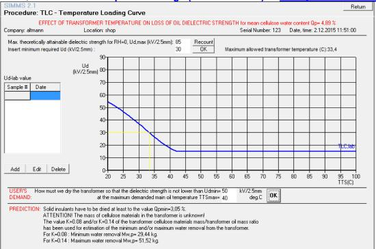
Simultaneously, based on the calculated TLC and allowed dielectric strength of oil (30 kV/2.5mm, horizontal yelow line), the maximum allowed temperature of the transformer (vertical yellow line : ca **33.4C**) is determined.
