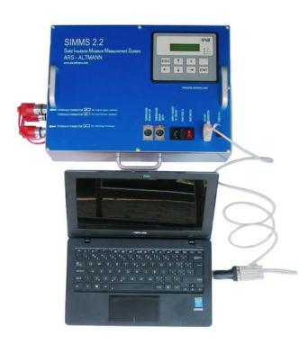
For the desired precision reading of the water content in the oil, the precise evaluation of the water content in oil (the Qw-value), the relevant evaluation of the water content in cellulose (the Qp-value) and the theoretical dielectric strength of oil (the Ud-value.
