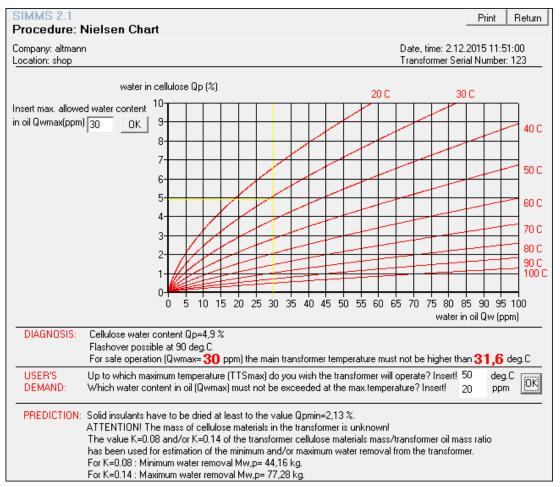
Diagnosis section then interprets the reading and calculates the averaged water content in cellulose (here Qp= 4.9%). Based on the entry of target value of water content in oil Qwmax = 30ppm and given water content in cellulose Qp = 4.9% then calculates the
