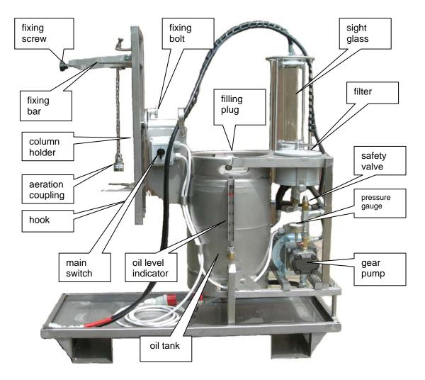
The column with a molecular sieve filling is fixed into a revolvable holder. Its upper and bottom part is connected to the washing system via two flexible hours, enabling its 180 grad rotation of the column. The gear pump forces the washing oil from oil tank into the upper part of the column, and dust contaminated oil from its bottom flows via sight glass and bulk filter back into the oil tank.
