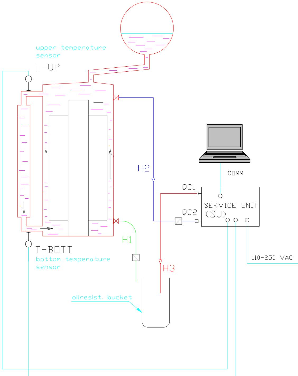
Fig. 5 Deaeration and flushing of outlet hose H2
