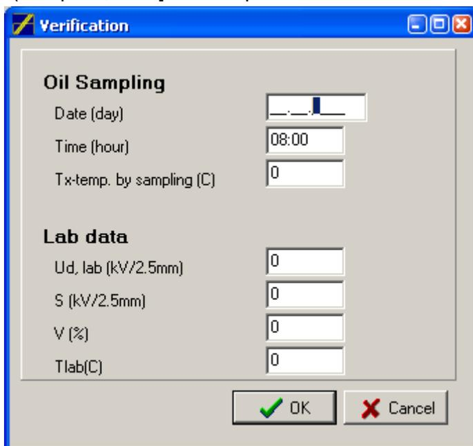
where the **Oil sampling** data ( Date, Time, Tx-temp by sampling) and the **Lab data** (Ud,lab-value, S.. Ud-deviation, V-deviation, Tlab-temp) can be easily entered.
