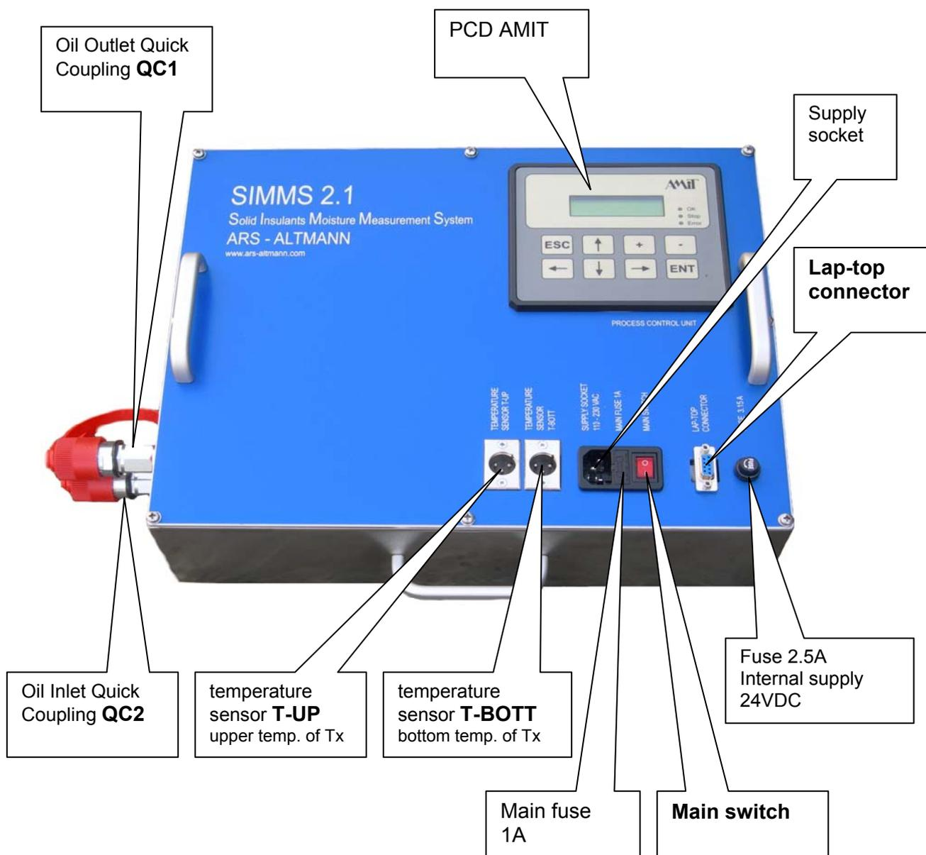
Fig. 2 The face-plate of the Service Unit (SU)
