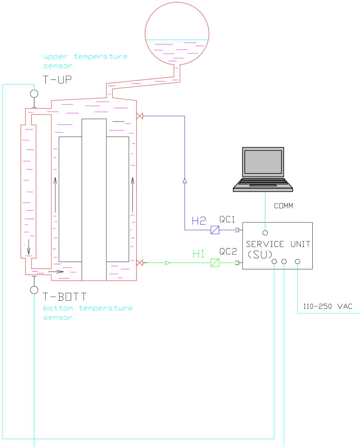
Fig. 6 Finalization of hydraulic interconnections of transformer and SU
