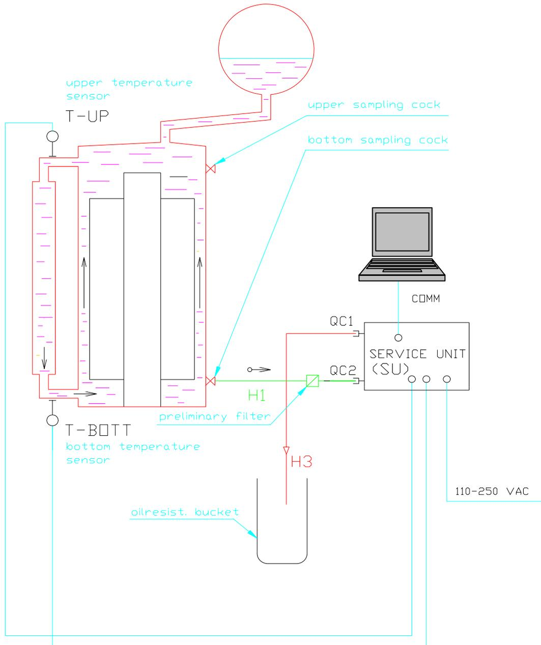
Fig. 4 Deaeration and flushing of inlet hose H1
