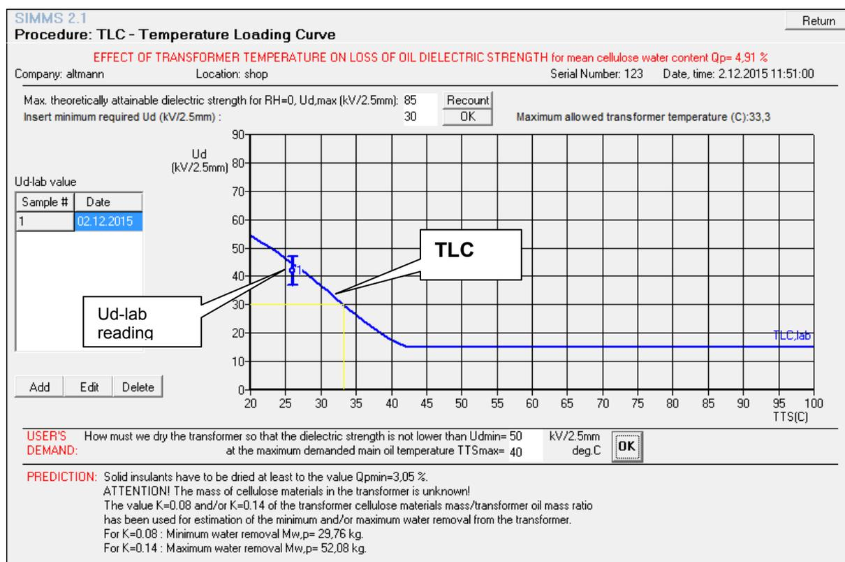
Simultaneously, based on the calculated TLC and allowed dielectric strength of oil (30 kV/2.5mm , horizontal yellow line), the maximum allowed temperature of the transformer (vertical yellow line : ca 33.4 C) is determined.
